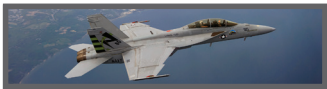
NAS Patuxent River did the first test flight of the Green Hornet, a bio-fueled F/A-18 jet.
